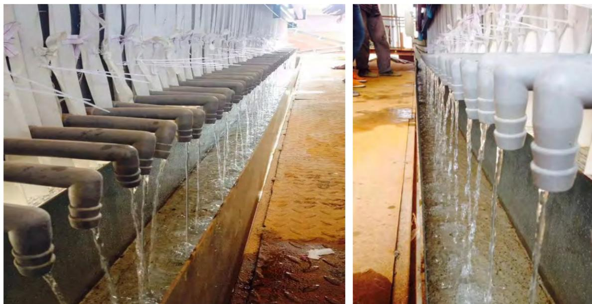
Filtrate that passes through filtration cloth is collected through collection pipe. After filtration process is finished, by pulling the filtration plates apart from each other, the sludge cake will fall down from those separation chambers and are then discharged to the final collection point.
