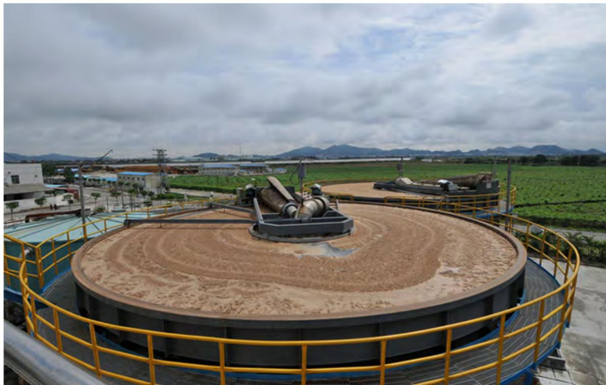
DAF clarifier purify wastewater by removing suspended solids, is a cost-effective alternative to conventional sedimentation clarification process, specially designed for high TSS wastewater, oily wastewater, paper mills backwater as well effluents from sugar, dairy, food, textile industries and tanneries.
