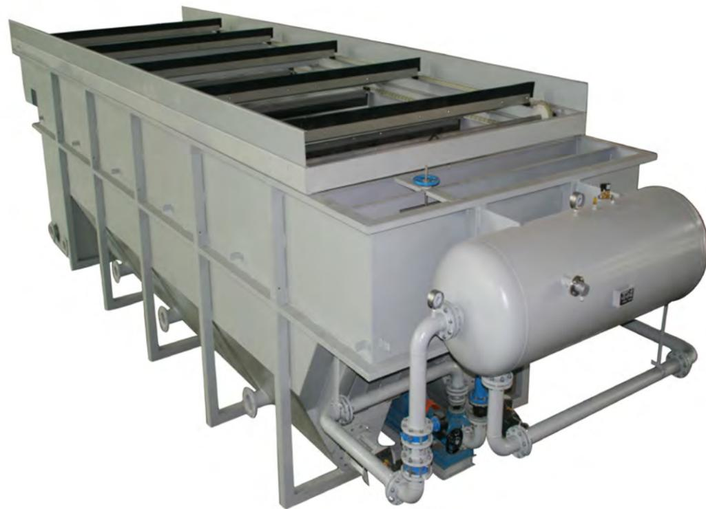
The feed water to DAF float tank is often (but not always) dosed with a coagulant (such as ferric chloride or aluminum sulfate) to coagulate the colloidal particles and/or flocculants to conglomerate the particles into bigger clusters.
