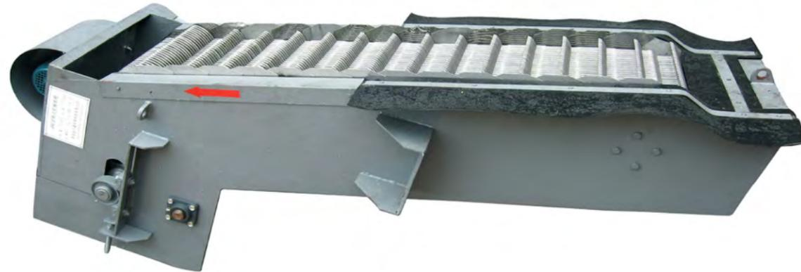
This automatic bar screen is mainly composed of electric motor, gearbox, steel frame, tooth rake, and transmission system. Electric motor and gearbox are mounted at the head of steel frame, together with driving sprocket and traction chains, forming the driving system.
