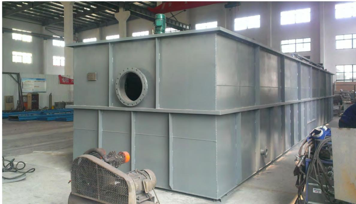
CAF Cavitation Air Flotation Machine is greatly different from DAF Dissolved Air Flotation Machine in its air dissolving method: One or several sets of CAF aerator(micro bubble generator) is installed in the aeration chamber of CAF machine. With the high speed rotation of impeller of CAF aerator under water, a vacuum zone is formed there and absorb the air above water surface into water and generate millions of micro bubbles.
