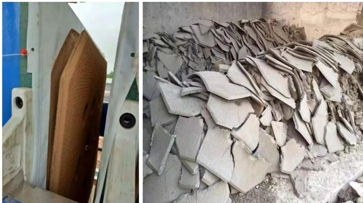
The slurry is fed to filtration chambers and the sludge cakes are accumulated. As the sludge cake becomes thicker, the filter resistance increases as well. When the separation chambers are full, the filtration process is stopped as the optimum pressure difference is reached.
